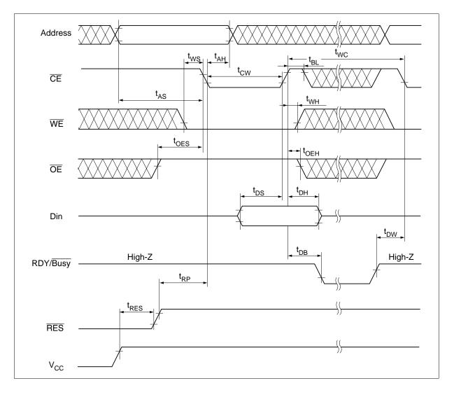
Byte Write Timing Waveform (2) (CE Controlled)
